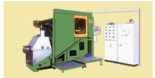
100 Bar High Pressure Die Casting machine from HADI GMBH, Austria costing Rs. 2.5 crores
